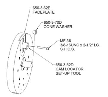
Locators: This fixture requires the use of locator sets, sized to fit individual engine blocks. These sets consist of (1) cam bearing bore locator, (1) #5 main bearing bore locator, and (1) #1 main bearing bore locator.
