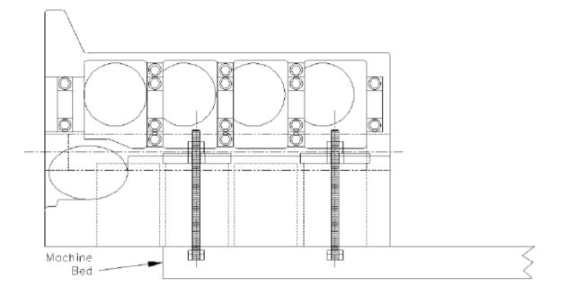
Screw the supplied 1/2-13 NC nuts on to the threaded rod and snug them up. Do not tighten them all the way at this point.
