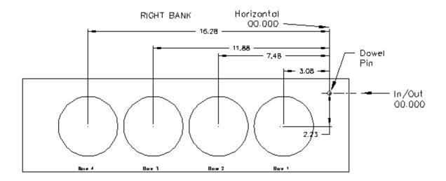
Select Left Locations and then Indicated. If you have programmed the blueprint locations into this program then press Copy Values and then Blueprint. This will cause the values from the Blueprint page to be copied into the Indicated page. This give you a starting point to indicate the individual cylinder from.
