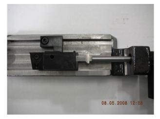
Slide the large diameter anvil up until it touches the end of the cutting tip of the tool holder. Tighten the set screw.
