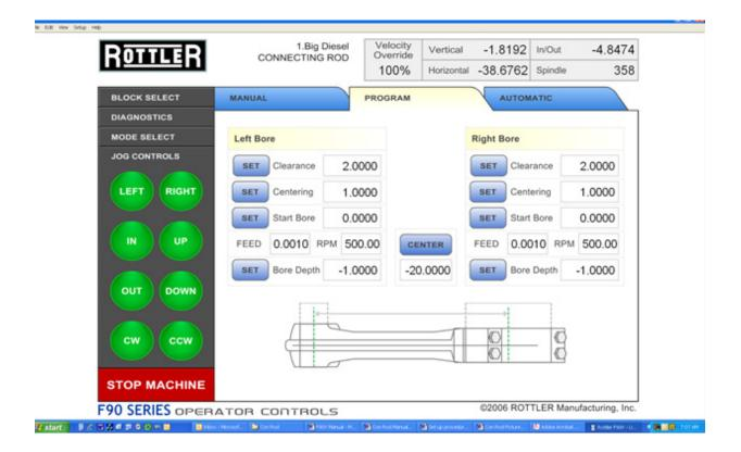
This screen is used to input all the parameters for boring both the big and small end of the rod plus setting positions for centering and measuring.
