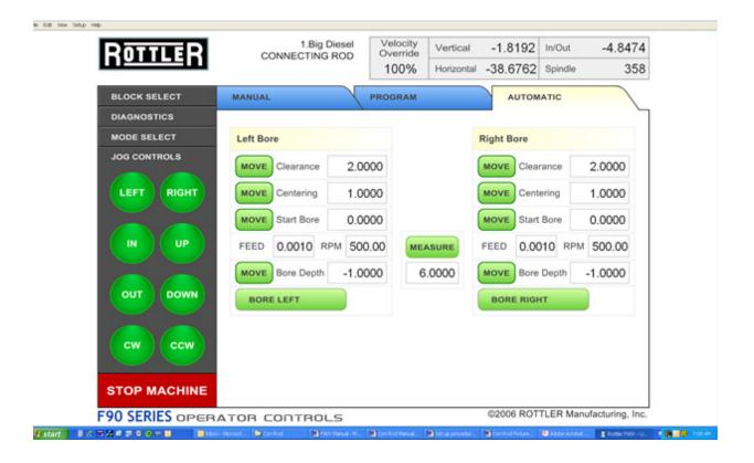
This screen is used to run programs such as bore right big end of the conrod. When the green buttons are touched, the machine will move to the position or start an automatic cycle.
