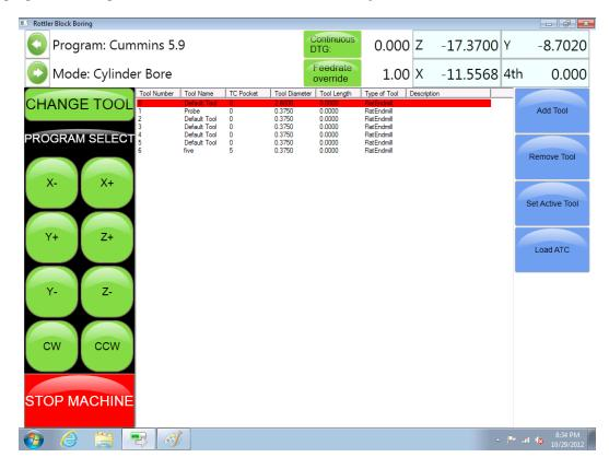
To set Tool Offsets you will need a fixed vertical reference point on the machine that does not change such as the head stock of the 4<sup>th</sup> axis or Performance Fixture.
