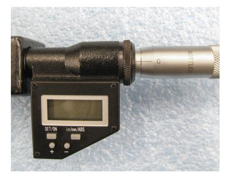
Turn the thimble until the '0' line on the thimble lines up with the vertical line nearest the spindle lock ring.
