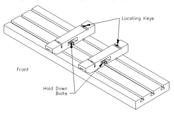
Select the 60 or 90 degree position for the fixture. Using a slow moving hoist, set the V6/V8 fixture onto the parallels.
