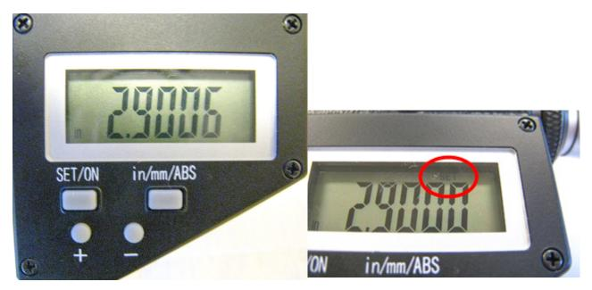
Press and hold the set/on button and the + or – button at the same time. "Set" will flash in the display. This places the micrometer in edit mode. (CAUTION: use a pencil tip or something similar to gently push the small round buttons - they are quite small and a bit delicate.)
