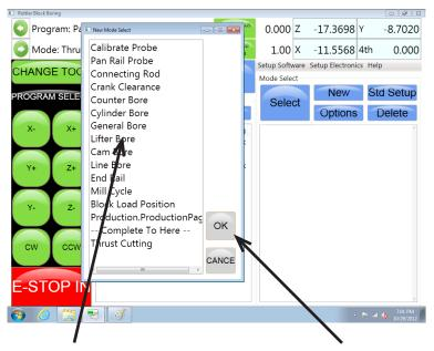
Select the operation you want to create and then press OK. This will place a general Bore operation under the Cylinder bore mode in the right hand section.
