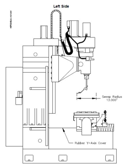
Loosen the four Spindle Main Bolts slightly. Using the Adjustment bolt on the right hand side of the spindle head, sweep the spindle to within +/- .0002 Left to Right. Do not worry about the Front to Back reading at this time as the Spindle Main bolts are not tight
