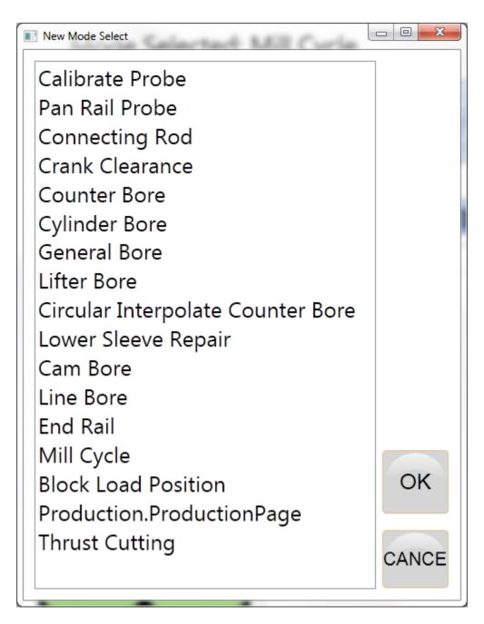
Click on the New button to view all of the available modes. This will take you to the Rottler program where the handwheel can be used. Highlight the Cylinder Bore mode and touch the OK button. This will bring up the Operation screen.
