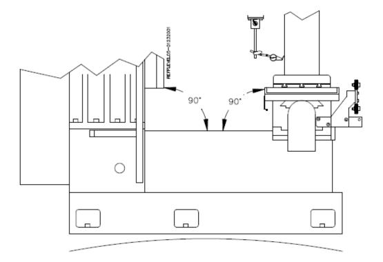
The arched line underneath the picture is illustrating the bow to the casting if the middle leveling bolts have too much pressure on them.
