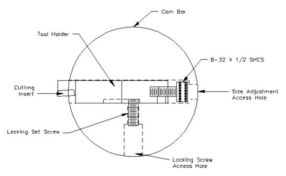
Once the size has been set, lock the set screw in the Cam Bar to secure the tool.
