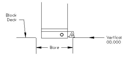
The zeros points for all axis have now been set. All the numbers entered from this point on will reference these zero positions. You are finished with the Set Zeros screen, select the next Tab to the Right.
