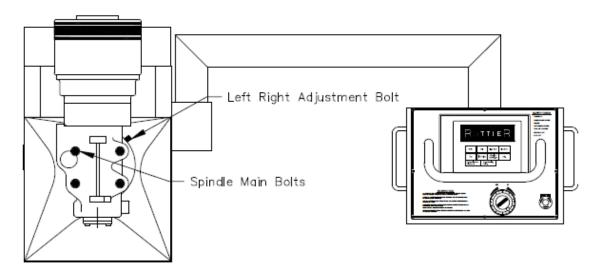
Check the Front to Back sweep it should be within .0005. If it is not, the Vertical gibs may need adjustment.
