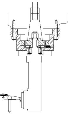
Put some pressure on the indicator. Using the In/Out handwheel move the indicator form one side to the other noting the amount of difference. Keep the indicator on that side of the head and rotate it half of the noted distance. Repeat this procedure until there is less than .0005" variance.
