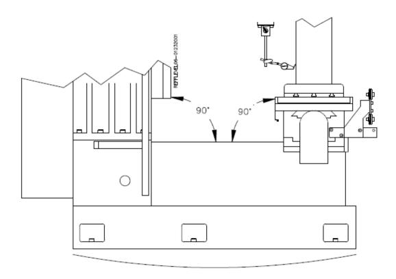
The arched line underneath the picture is illustrating the bow to the casting if the middle leveling bolts have too little pressure on them.
