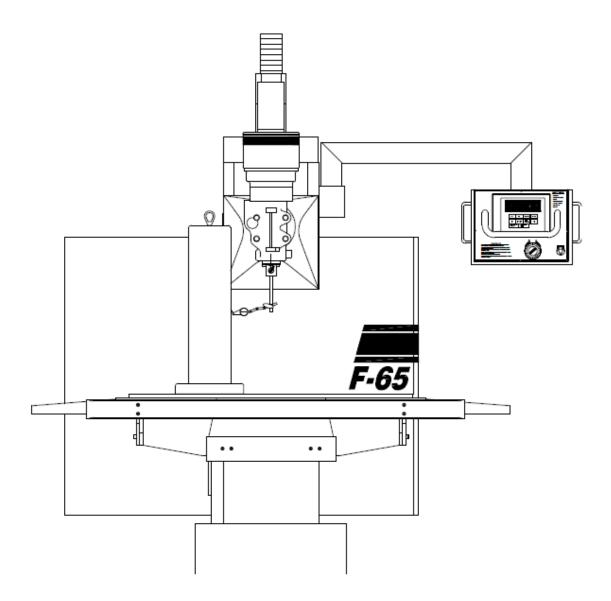
Put about .010" pressure on the indicator. Run the vertical throughout its full travel. The runout should not be more than .0005. If the runout is more than this, check the table top as well as the bottom of the alignment cylinder for burrs or debris.
