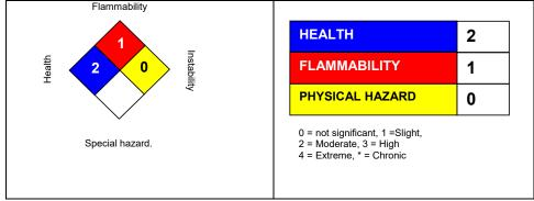
NFPA Flammable and Combustible Liquids Classification Combustible Liquid Class IIIB
