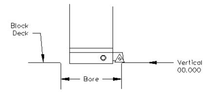
The zeros points for all axis have now been set. All the numbers entered from this point on will reference these zero positions. You are finished with the Set Zeros screen, select the next Tab to the Right, Vertical Stops.
