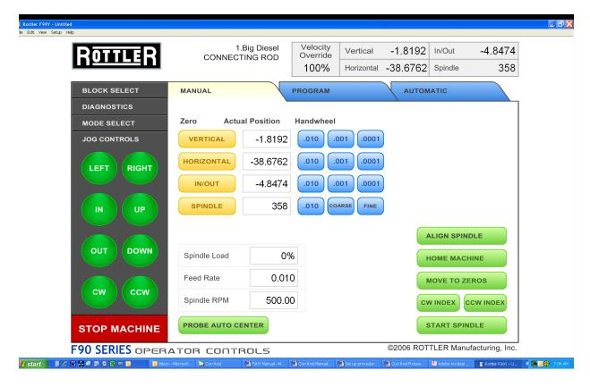
This screen is used to set the center of the conrod to be bored and a vertical height reference for the cutterhead and boring tool to be used.
