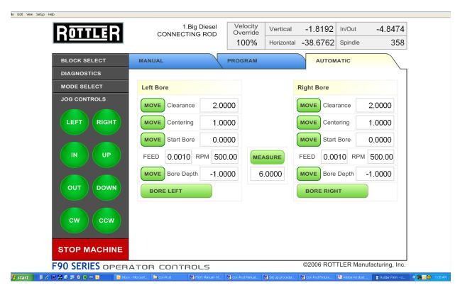
This screen is used to run programs such as bore right big end of the conrod. When the green buttons are touched, the machine will move to the position or start an automatic cycle.
