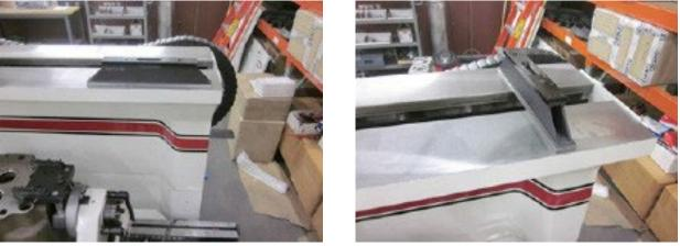
Use the level on the upper float surface, level the machine as precisely as possible, front to back and side to side.
