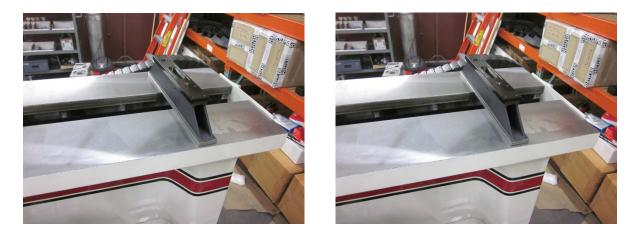
Level the machine using the upper float surface for reference as shown in the images above. it is recommended to level the machine in the front to back direction and then side to side. The machine should be level within .0001"/1' as visualized through the levels viewing glass and graduation lines. Check both directions after adjusting and before tightening the lock nuts to ensure that the machine is indeed level.
