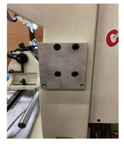
Step 2: Remove the 4 bolts that secure the bottom cover located on the bottom of the sharpener unit
