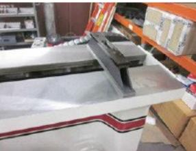
Use the level on the upper float surface, level the machine as precisely as possible, front to back and side to side.
