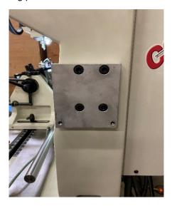
Step 2: Remove the 4 bolts that secure the bottom cover located on the bottom of the sharpener unit
