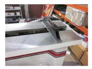
Use the level on the upper float surface, level the machine as precisely as possible, front to back and side to side.
