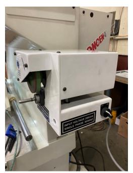
Step 5: Wire the sharpener by running the power cable through the side of the cabinet and over to the breaker in the electrical cabinet. The sharpener is wired by attaching the red and black power leads to the T1 and T2 terminals on the lower part of the breaker as shown in the figure below. The green and yellow ground cable can be connected to any open ground terminal in the terminal block behind the breaker.
