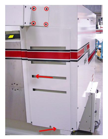
For a finished look push natvar covered wires to the left through slots in sheet metal and push natvar up from the bottom right.
