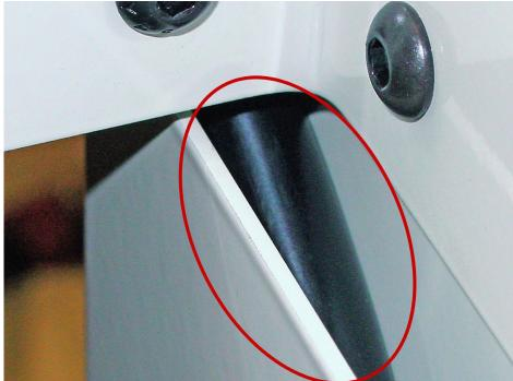
(Make sure you are not pinching any wires) Then mount the screen enclosure bracket to the machine with 4 each supplied  $1/4-20 \times 1/2$ " BHCS.
