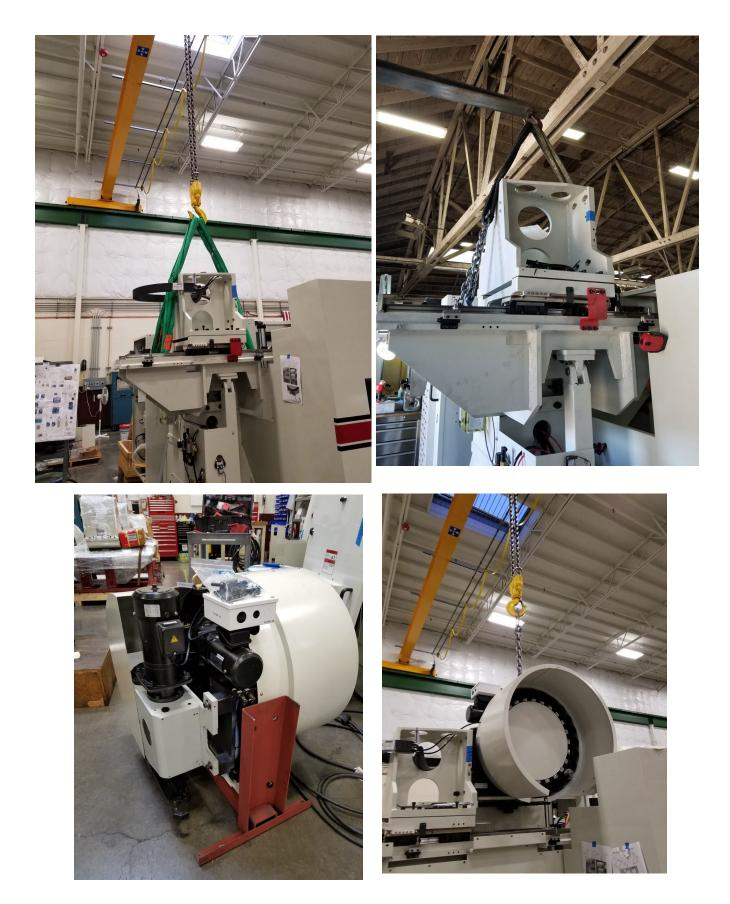
\_\_\_Install machine with jack pads under jacking bolts. Refer to the Machine Installation section in the manual for proper uncrating and leveling instructions.
