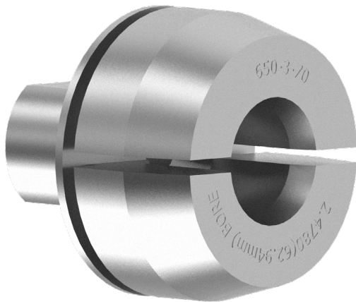
650-3-70 Locator, Cam, Expanding (2.4780 - 2.4795" bore) (62.94 - 62.98mm)
