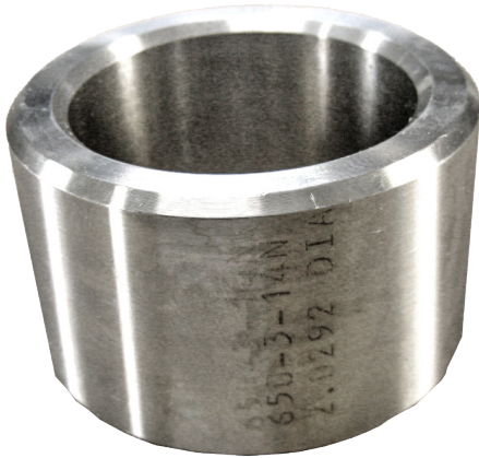
650-3-14N Locator, Cam (2.0297 - 2.0317" bore) (51.55 - 51.60mm)
