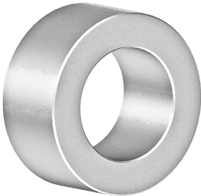
502-1-47V Locator, Main Bearing (3.3854 - 3.3862") (85.989 - 86.009mm)
