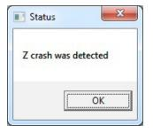
If there is an occurrence of an interference point being detected the machine will stop and a pop up screen will appear on the screen.
