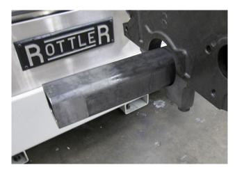
Use an appropriate method to place the block on the riser parallels with the front of the block facing left or away from the control pendent.
