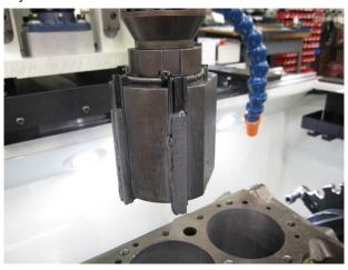
Remove hone head and clean the abrasive. Closely look at abrasive to determine if there is a solid line of contact the entire length of abrasive. If there is not a solid line contact on either the leading or trailing edge of abrasive then repeat the process again.
