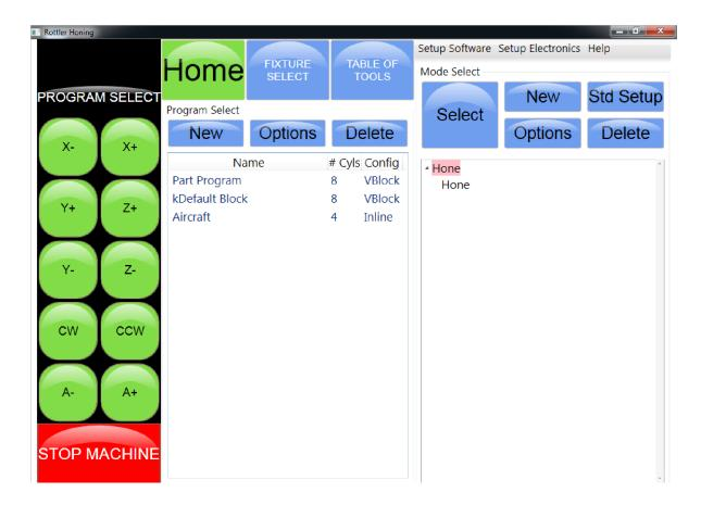
This is the Home screen. Using the jog buttons touch the X+ button to move the carriage to the right side of the machine. Touch the Z+ button to raise the spindle all the way to the top. Now the machine is in its block loading position. Engage the E-STOP by pressing the red E-STOP switch.
