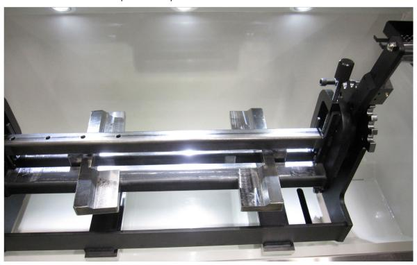
Place the clamp bar tube through the main bore of the block. Be certain that the machined flats at the end of the clamp bar tube are in a vertical position.
