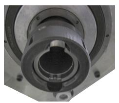
The hone head will have the standard locking tabs on the mounting adaptor and a drive coupler for adjusting the stones. When mounting the hone head, it will be necessary to align the drive coupler with its
