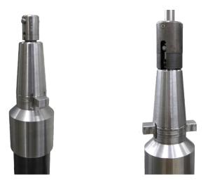
Due to design the nut will continue tighten during use. When it comes time to change or remove the hone head it may become so tight that the release wrench will be needed to loosen the locknut. Turn locknut clockwise to release the hone head.
