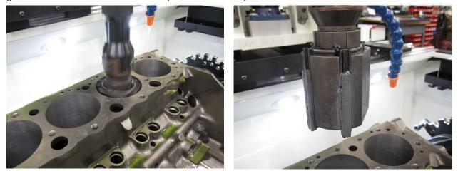
Remove hone head and clean the abrasive. Closely look at abrasive to determine if there is a solid line of contact the entire length of abrasive. If there is not a solid line contact on either the leading or trailing edge of abrasive then repeat the process again.
