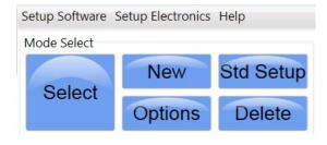
Setup Software and Setup Electronics menu titles will open new options menus. These are mostly used for machine setup at the factory or for service. There are 2 options that an operator can select if needed and will be explained further on.
