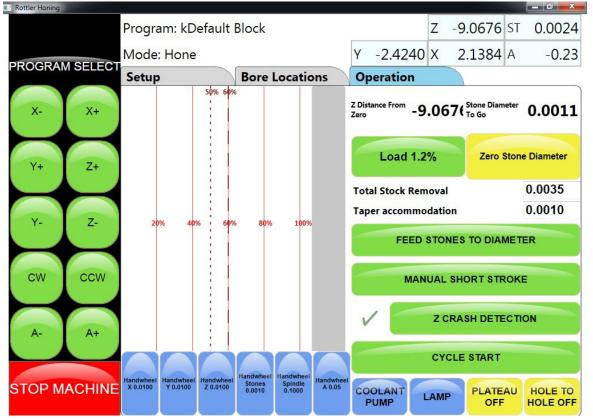
This is the screen where the honing operation will be run from. At the top under the Operation Tab are 2 readouts. The first is Z Distance From Zero. This reading shows the location of the spindle from the zero point. The second is Stone Diameter To Go. This readout shows how much the stones must still feed out to reach the Total Stock Removal setting.
