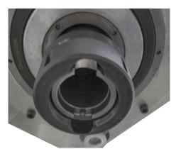
The hone head will have the standard locking tabs on the mounting adaptor and a drive coupler for adjusting the stones. When mounting the hone head it will be necessary to align the drive coupler with its receiver inside the drive spindle. Once they are aligned the adaptor tabs will fit into the receiver slots. The tabs will activate the release pin and the locknut will automatically turn to lock the hone head in place.
