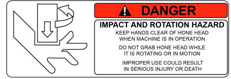
Honing - Do not engage rotation power when hone is out of a cylinder.
