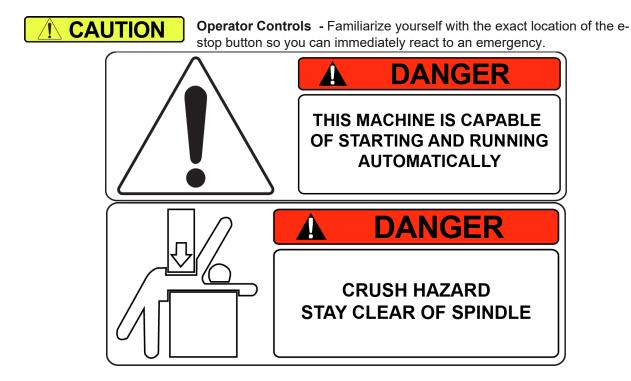
Keep clear of spindle when working in tank area. Spindle can drop if there is a failure in the machine. Move spindle out of work area when changing blocks or fixtures.
