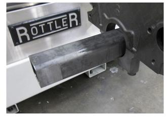
Use an appropriate method to place the block on the riser parallels with the front of the block facing left or away from the control pendent. Take care to align the clamp tube with the
