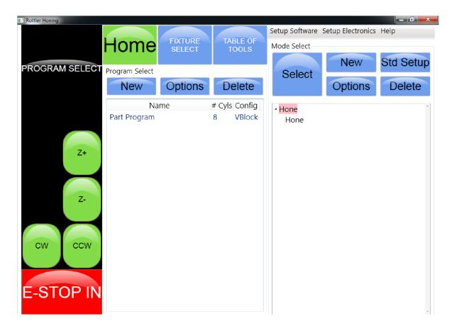
This is the Home screen. Using the jog buttons touch the X+ button to move the carriage to the right side of the machine. Touch the Z+ button to raise the spindle all the way to the top. Now the machine is in its block loading position. Engage the E-STOP by pressing the red E-STOP switch.
