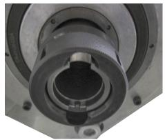
The hone head will have the standard locking tabs on the mounting adaptor and a drive coupler for adjusting the stones. When mounting the hone head it will be necessary to align the drive coupler with its receiver inside the drive spindle. Once they are aligned the adaptor tabs will fit into the receiver slots. The tabs will activate the release pin and the locknut will automatically turn to lock the hone head in place.
