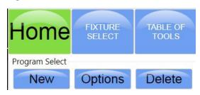
The Home button is use to index the hone head when it is installed on the machine. FIXTURE SELECT, and TABLE OF TOOLS buttons are not used on the H85A.
