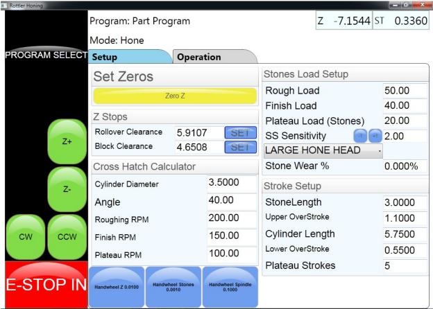
At the top of the screen you will see the block and process that was selected. In the upper right section there is a readout of current location of the different axis's. *All readings are plus or minus from the zero set points.* ( The A axis readout in this case is the 4<sup>th</sup> axis and will only show a reading if the optional auto rotate fixture is installed )
