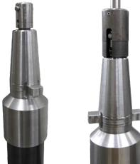
head it may become so tight that the release wrench will be needed to loosen the locknut. Turn locknut clockwise to release the hone head.
