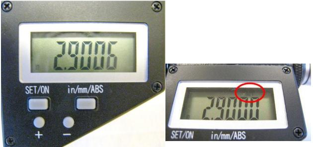
Press and hold the set/on button and the + or – button at the same time. "Set" will flash in the display. This places the micrometer in edit mode. (<u>**CAUTION**</u>: use a pencil tip or something similar to gently push the small round buttons - they are quite small and a bit delicate.)
