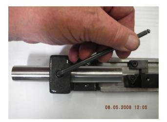
Back the digital micrometer shaft off, then bring it up to touch the tool holder and recheck that the numbers in the display are the same as the numbers previously shown.
