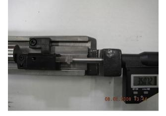
The micrometer is now set up for use with this cutter head.
