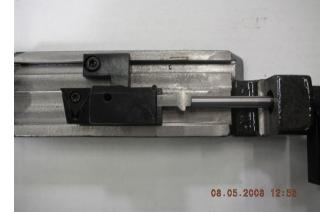
Slide the large diameter anvil up until it touches the end of the cutting tip of the tool holder. Tighten the set screw.
