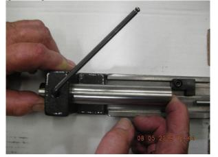
Place the tool holder used to bore the hole into the micrometer frame. Slide the location nub on the back of the tool holder gently up against the end of the digital micrometer shaft.
