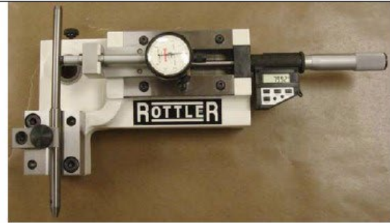
MEASURE VALVE STEM AND PILOT DIA.
