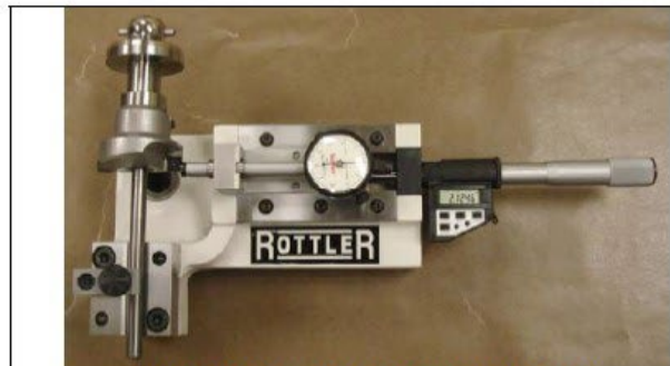
SET BORING INSERT FOR HOUSING DIA.
