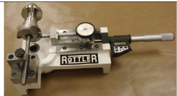
SET BORING INSERT FOR HOUSING DIA
