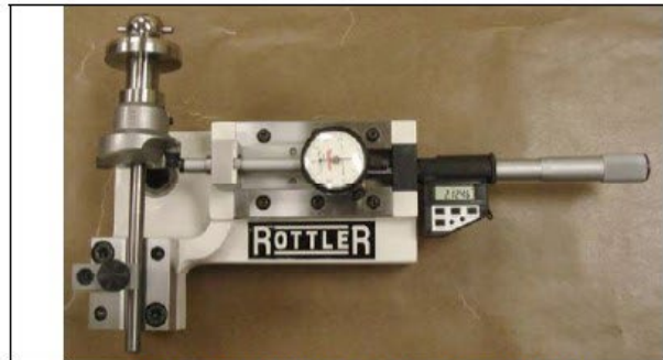
SET BORING INSERT FOR HOUSING DIA.
