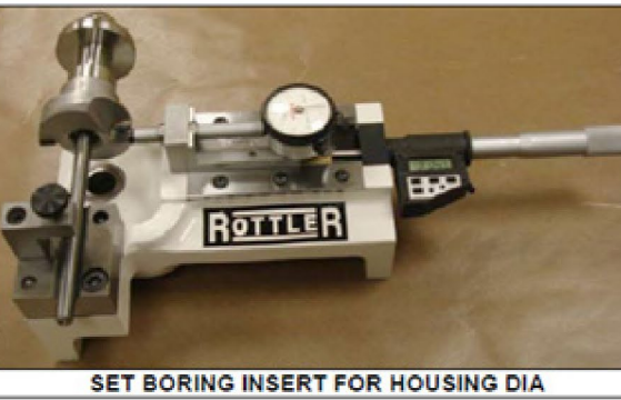
SET BORING INSERT FOR HOUSING DIA WITH TRIANGLE
