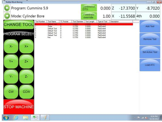
To set Tool Offsets you will need a fixed vertical reference point on the machine that does not change such as the head stock of the 4<sup>th</sup> axis or Performance Fixture.
