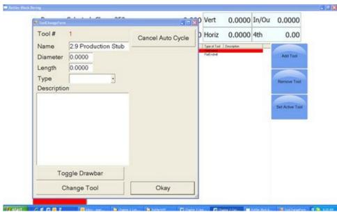
This window will open when the machine does an automatic tool change. This will be discussed in Chapter 3 Operating Instructions. After you press OK another window will open. This is a Warning Dialog box to inform the operator of the possibility of the spindle start if the tool change is done in an automatic program. Press OK.
