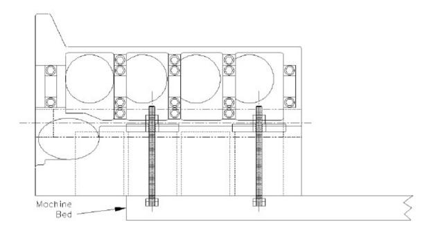
Screw the supplied 1/2-13 NC nuts on to the threaded rod and snug them up. Do not tighten them all the way at this point.
