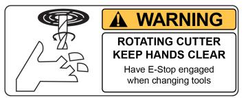
**Machining** – Eye protection must be worn during all operations of the machine. Hands must be kept completely away from the cutter head. All chip guards must be in position during machine operations.
