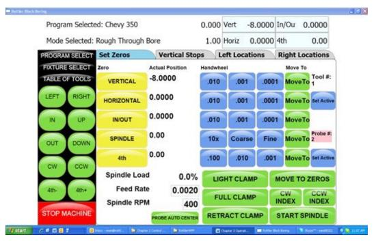
If you attempt to run the Probing Cycle with the Tool # active the machine will automatically move to the Tool Change clearance position and open the Tool Change Window so you can change the tool and vise versa.
