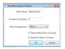
Pressing OK will result in the Block Model being inserted into the left hand side of the screen.
