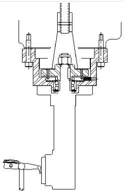
Put some pressure on the indicator. Using the In/Out handwheel move the indicator form one side to the other noting the amount of difference. Keep the indicator on that side of the head and rotate it half of the noted distance. Repeat this procedure until there is less than .0005" variance.
