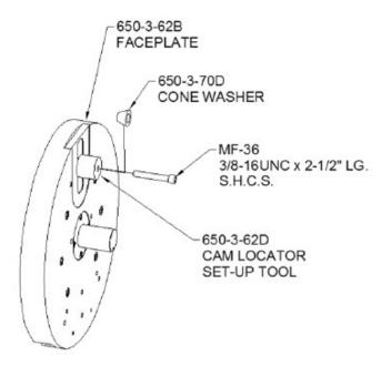
Locators: This fixture requires the use of locator sets, sized to fit individual engine blocks. These sets consist of (1) cam bearing bore locator, (1) #5 main bearing bore locator, and (1) #1 main bearing bore locator.
