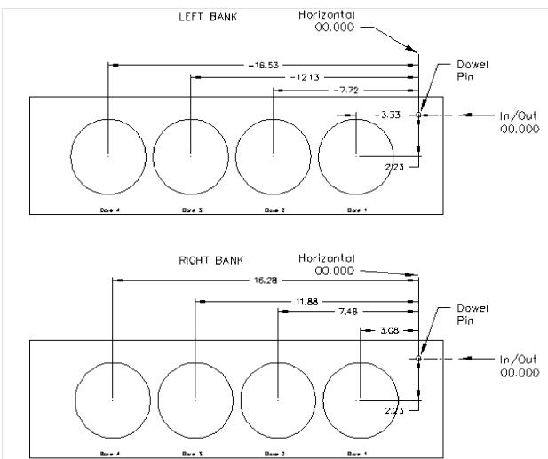
Select Left Locations and then Indicated. If you have programmed the blueprint locations into this program then press Copy Values and then Blueprint. This will cause the values from the Blueprint page to be copied into the Indicated page. This give you a starting point to indicate the individual cylinder from.
