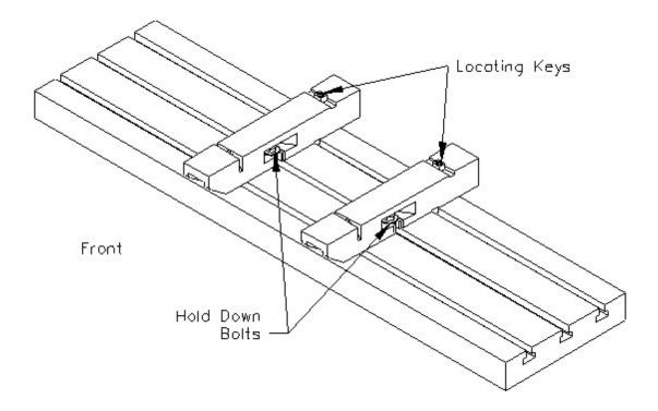
Select the 60 or 90 degree position for the fixture. Using a slow moving hoist, set the V6/V8 fixture onto the parallels.
