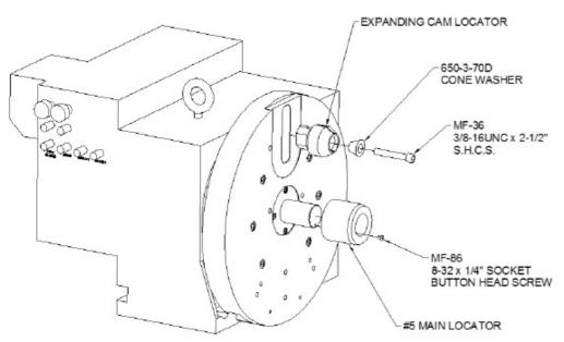
CAM AND MAIN LOCATOR INSTALLATION
