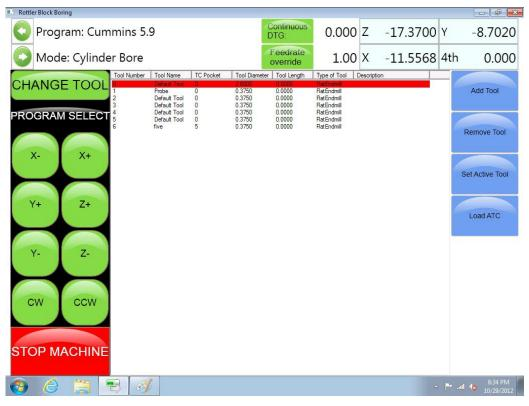
The Table of Tools comes with Tool 0 installed with no offset amount. Tool 0 will remain tool 0 with no offset always. Tool 0 will be set active when you are using programs that do not require tool offsets.
