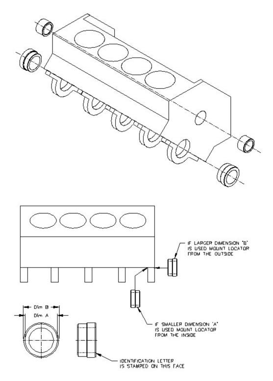
Note: Each locator covers two bearing diameters ('A' and 'B'). The unused diameter <u>MUST</u> be placed <u>INSIDE</u> the block to prevent interference with the Index plates.
