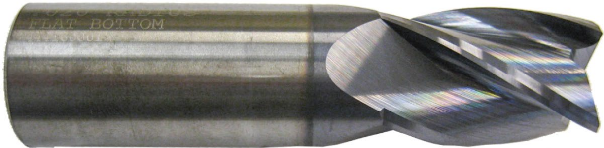
650-2-43F Four Fluted End Mill, 3/4" (19.05mm) x 4.00" (101.4mm)
