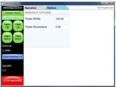
**Finish RPMs** default value is 125. When the machine reaches the Finish Cutting Depth the spindle RPMs change to this speed, rotate the number of times set by the Finish Revolutions parameter and index the tool to the index position. The operator can change this value to any value he chooses.
