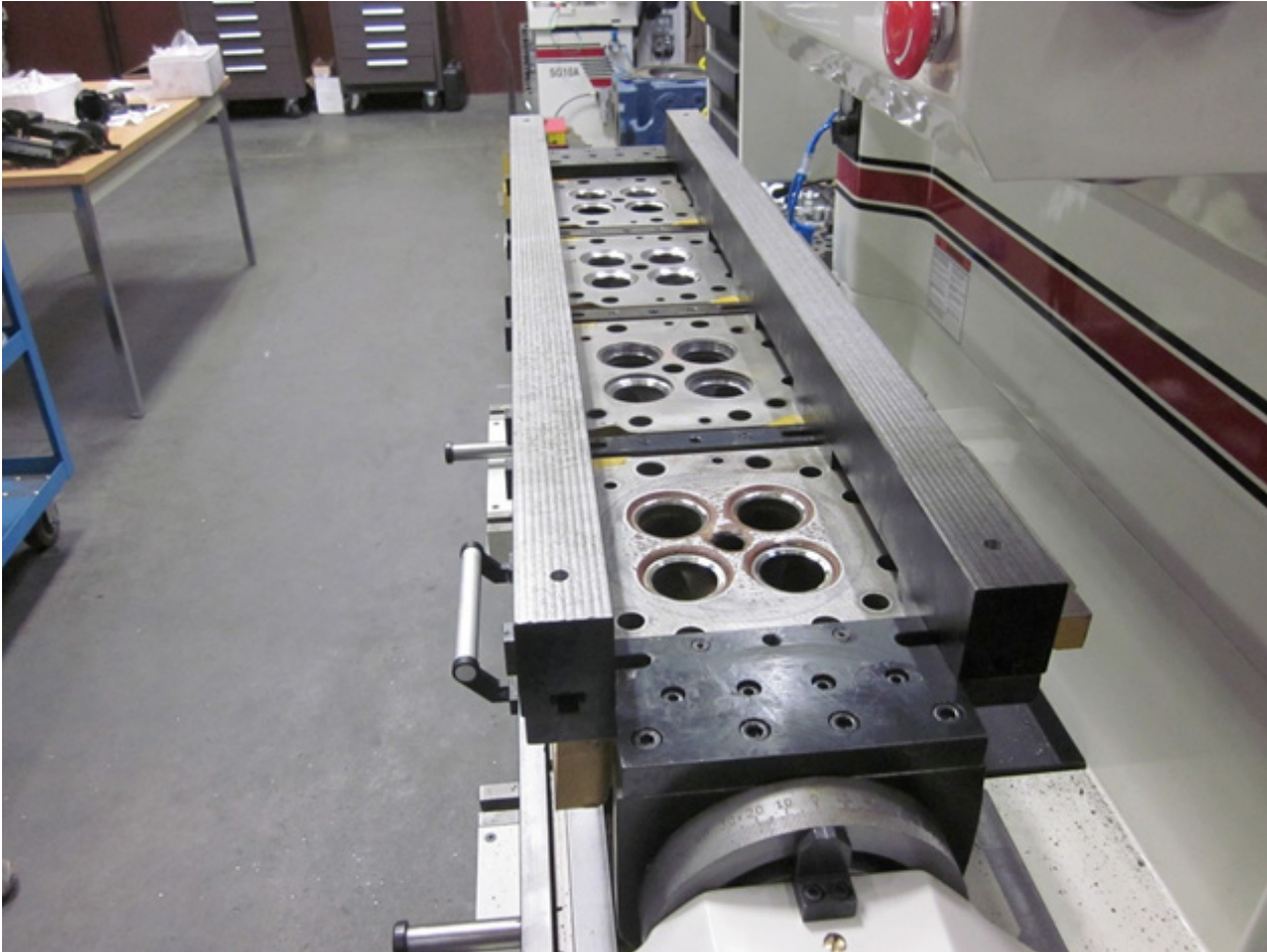
4 Cat 3500 heads in cutting position
