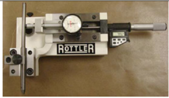
MEASURE VALVE STEM AND PILOT DIA.
