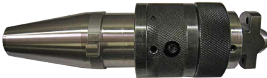
RBHAR40UPT and UPT5400SH assembled. Note one of the two screws (center) that locks them together
