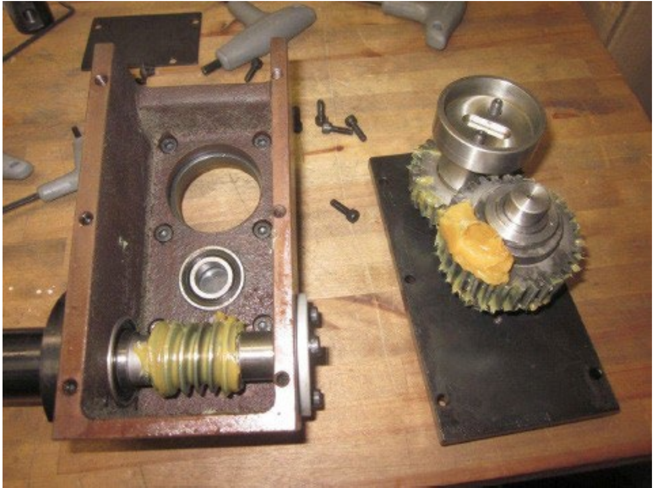
Take mount plate from gearbox and place on fixture
