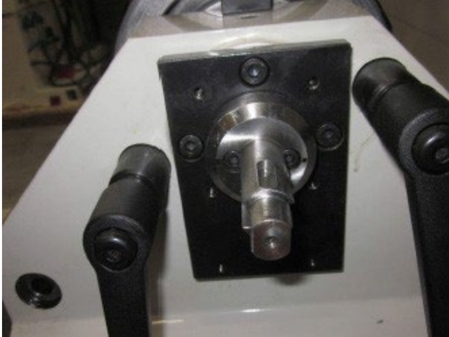
Bolt gearbox housing to mount plate on fixture
