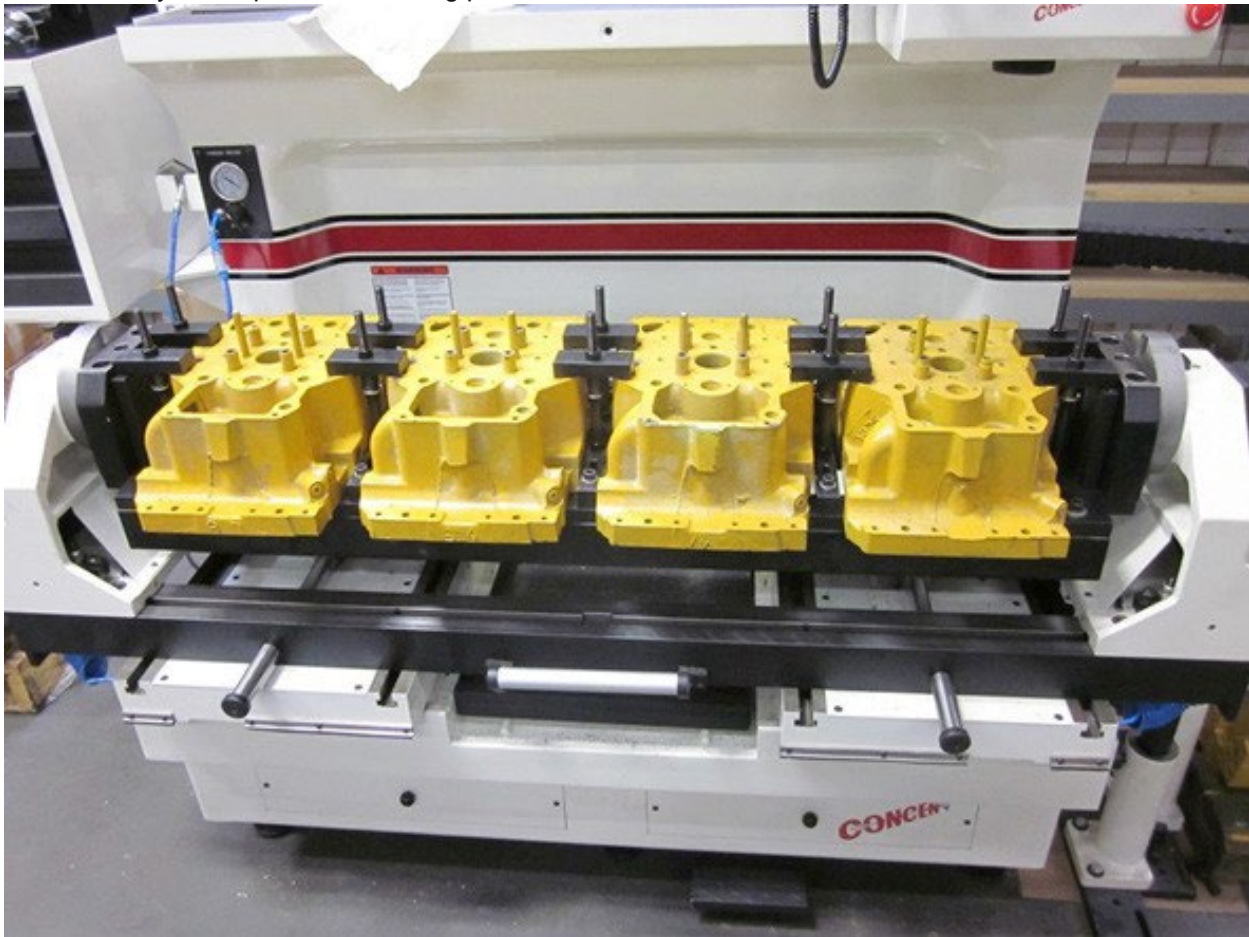
4 Cat 3500 heads in loading position. 4 Cat 3500 heads in cutting position
