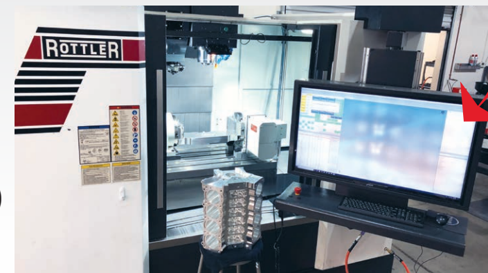
Complete V8 block from 268lbs to 38lbs (122kg to 17.3kg)
