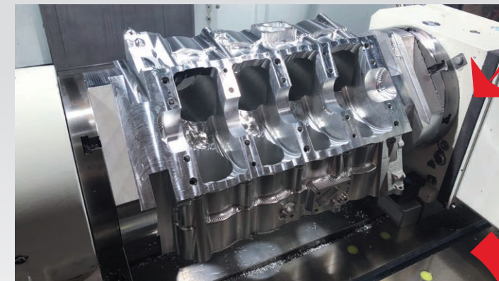
Advanced stage of billet machining into a V8 Block
